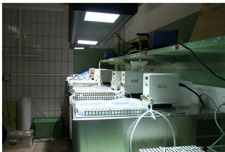
Fig. 3 Thermal treatment. Fucus vesiculosus germlings cultured in plastic boxes containing aerated seawater placed into water baths).
